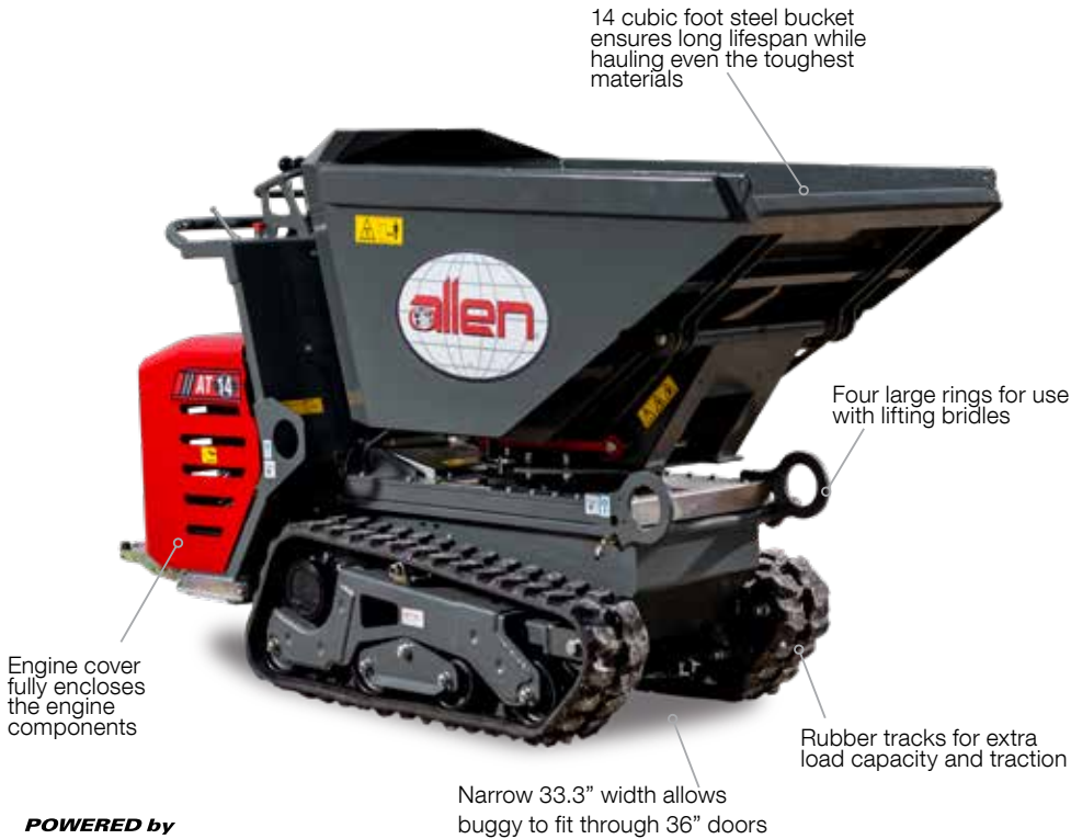
Swivel design allows bucket to turn 90° in either direction from center.
