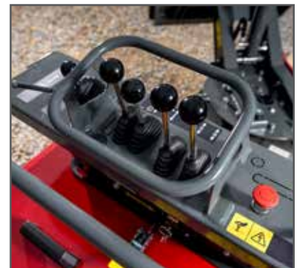
Two servo levers control the direction of the machine, and they automatically reset to stop in case of emergency.
