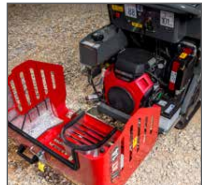
Engine cover folds back to provide convenient access to the engine, gasoline tank, battery, and filters.
